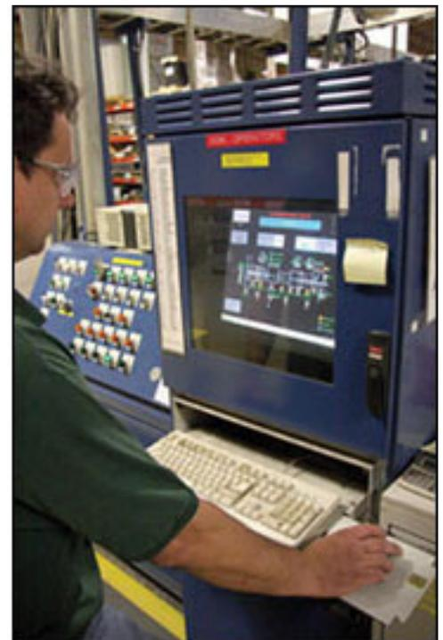
An automated metal punch press line uses a host CNC to command nine presses that complete finished drawers in about seven seconds.
