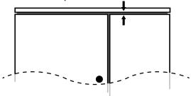
To improve horizontal gap, loosen the Torx screws only enough to slide the hinges. Do not remove the screws completely. Carefully slide the doors up or down until the horizontal gap is uniform. When properly aligned, tighten the screws.
