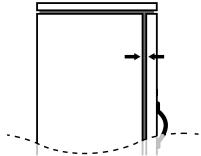
To improve the door gap at the side of the cabinet, loosen the side gap Phillips hinge screw and slide the hinge back to close the gap, or forward to increase the gap. Do not remove the screw. Tighten when finished.
