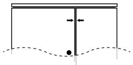
To improve the vertical gap, adjust the Phillips screw. Tightening the screw will pull the door toward the center of the cabinet. Loosening the screw will pull the door toward the outside edge.
